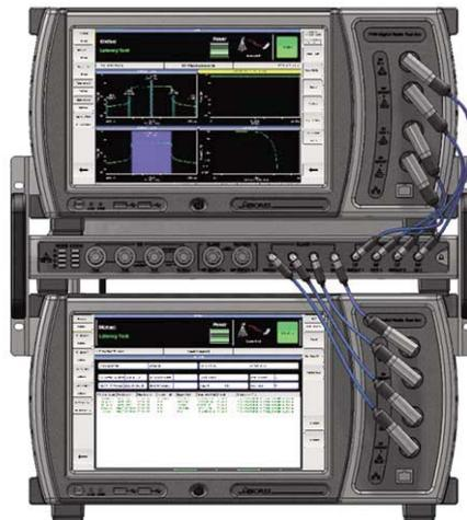
Using this setup allows UE Cat 6 maximum data rates to be tested, with the full 301.5 Mbps downlink and 50.024 Mbps uplink physical layer rates possible simultaneously using IPv4 and IPv6, TCP and UDP, with multiple connections supported. Remote API calls are provided to support automated testing, and detailed logging is available for fault diagnosis. The user can control the activation and de-activation of the secondary cell and can divert traffic through the PCell, SCell or both, as required.
